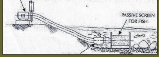
Passive screens are self-cleaning, only allowed on diversions less than 3 cfs. Sweep velocity must be higher than intake velocity.
